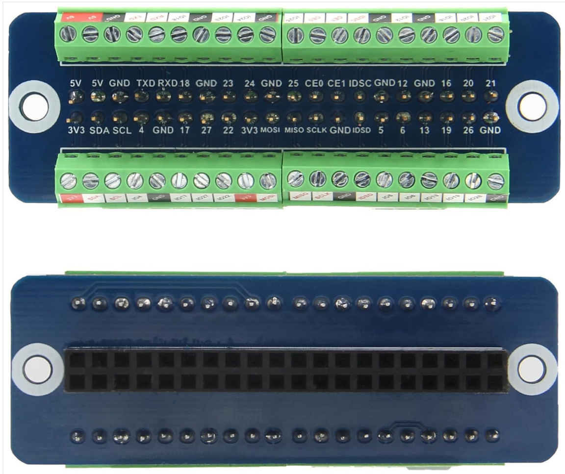
Figure 6.1: Top view of the G469 board showing clear pin labels for easy identification.
