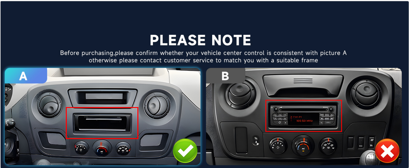
Figure 2: Dashboard compatibility. Ensure your vehicle's center console matches configuration 'A' (left side, with a single DIN opening) for proper installation. Configuration 'B' (right side, with a factory radio) is incompatible without modifications.
