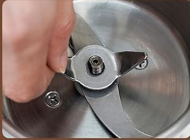
Figure 6.2: Step-by-step guide for replacing the grinding blade.
