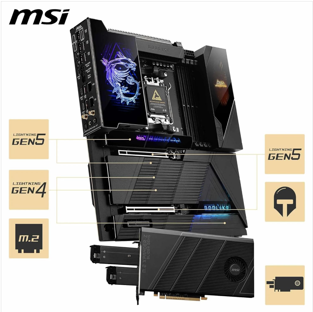
Figure 2: Overview of the M.2 slots on the MSI MEG X870E GODLIKE motherboard, highlighting the PCIe Gen5 and Gen4 compatibility, and the M.2 XPANDER-Z SLIDER GEN5 expansion card.
