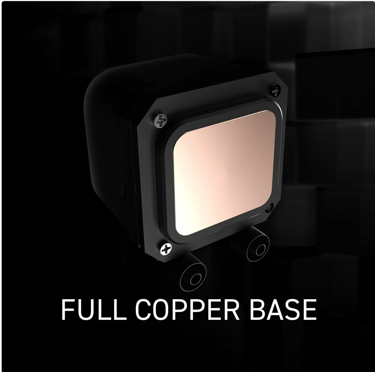
Figure 2: Full copper base of the cold plate for optimal heat transfer.
