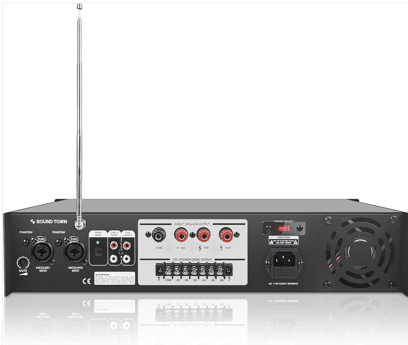
Figure 2: STCA600-6Z Amplifier Rear Panel. Connections include XLR/TRS combo MIC inputs with phantom power, RCA line inputs, direct speaker outputs (4-16 ohm), and 70V/100V speaker zone outputs with common ground.
