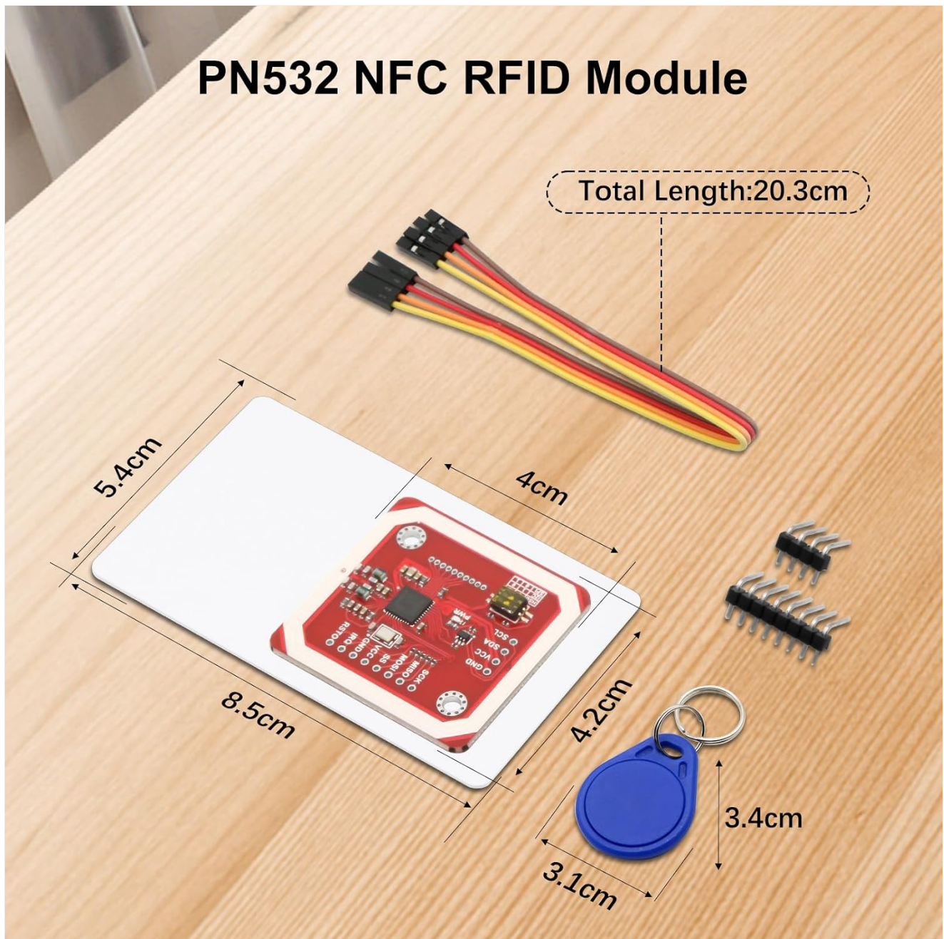
Image: Overview of the PN532 NFC RFID Module V3 Kit components, including the module, white card (5.4cm x 8.5cm), key fob (3.1cm x 3.4cm), and a 20.3cm cable. The module itself measures 4cm x 4.2cm.
