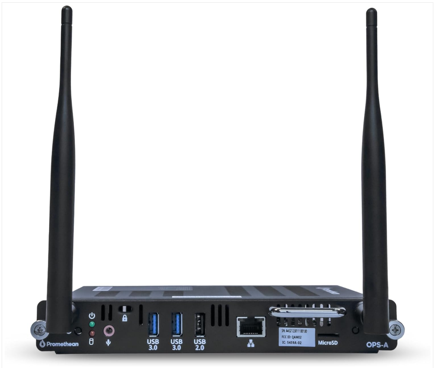
Figure 1: Rear view of the Promethean OPS-A module, showing USB ports, network port, and antenna connectors.
