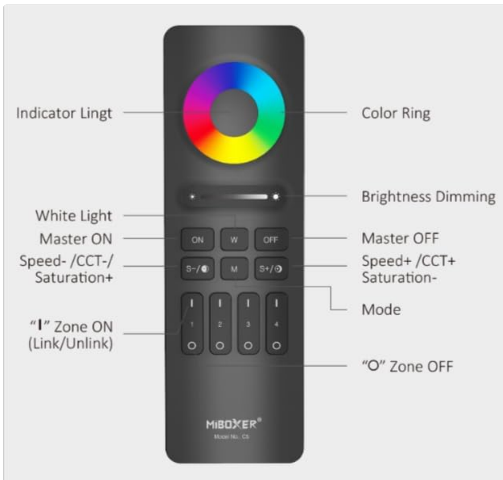
Figure 2: MiBOXER C5 Remote Button Diagram. This diagram illustrates the various buttons and their corresponding functions on the remote control.
