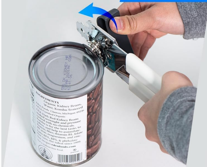
3. Turn the knob to cut the can lid completely along the edge of the can wall
