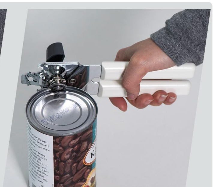
2. Squeeze the handles so the blade opens a cut in the can lid
