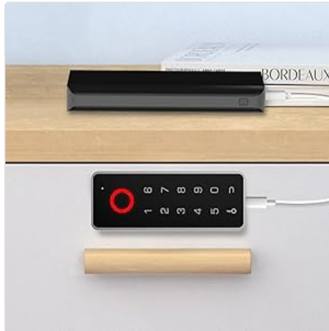
Figure 10: Connecting external power for emergency unlocking.
