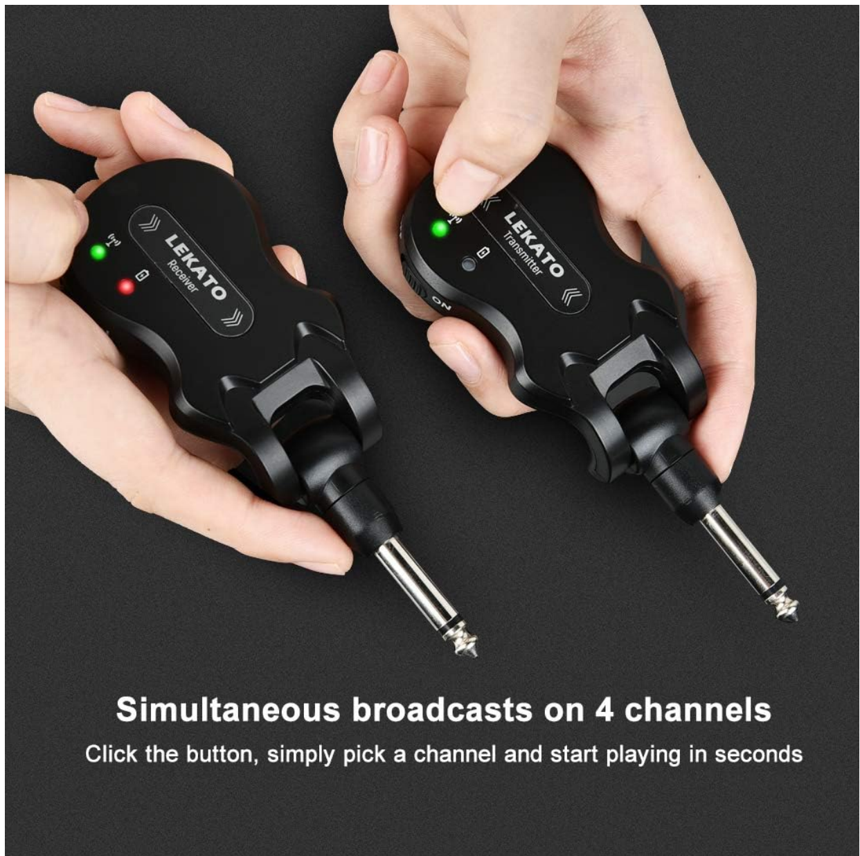
Figure 4.3: Demonstrating the simultaneous press of the signal key for pairing the guitar system.
