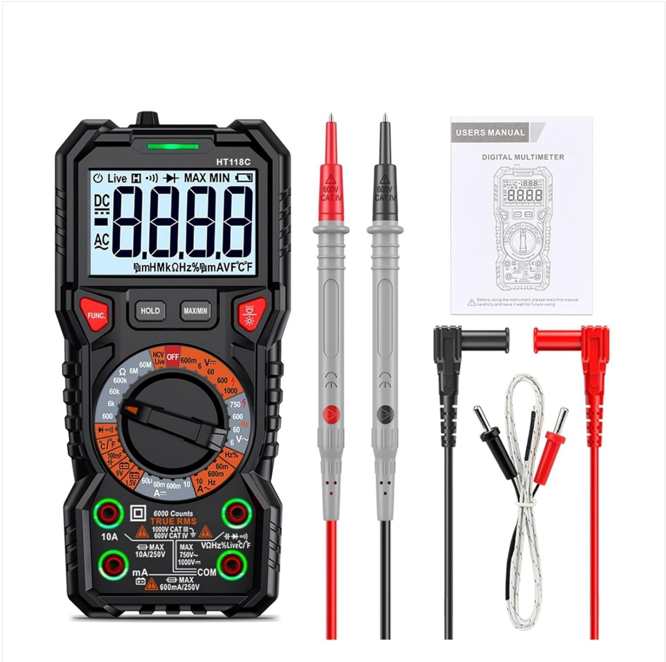
Figure 3.1: Contents of the HT118 package, including the multimeter, test leads, and user manual.
