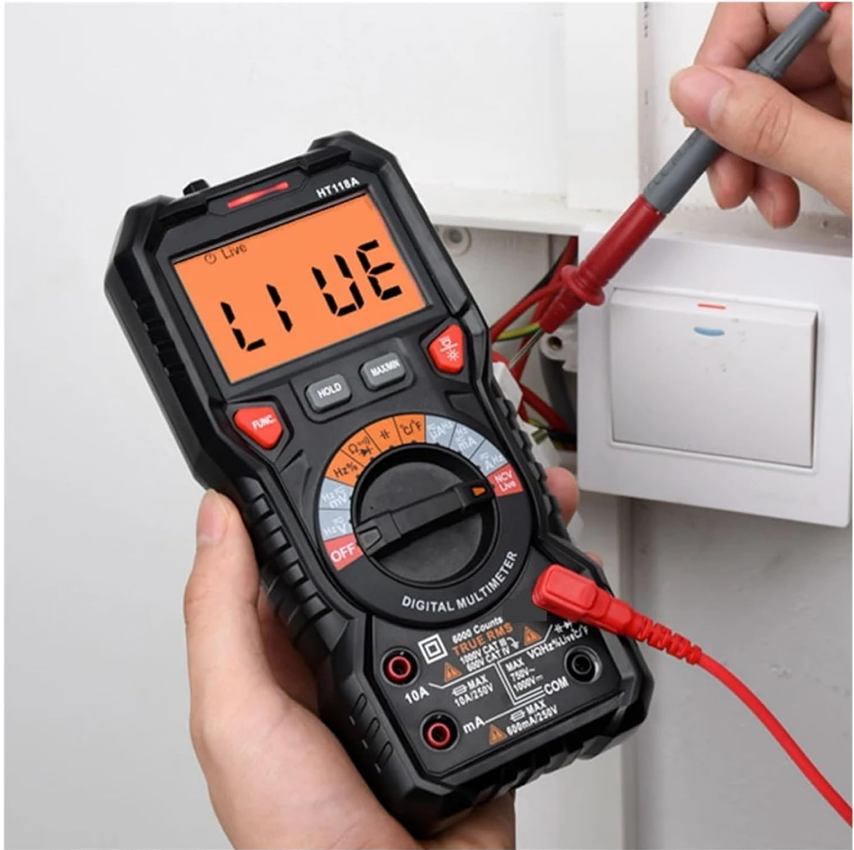
Figure 6.2: The HT118 multimeter in NCV mode, detecting voltage near an electrical outlet.
