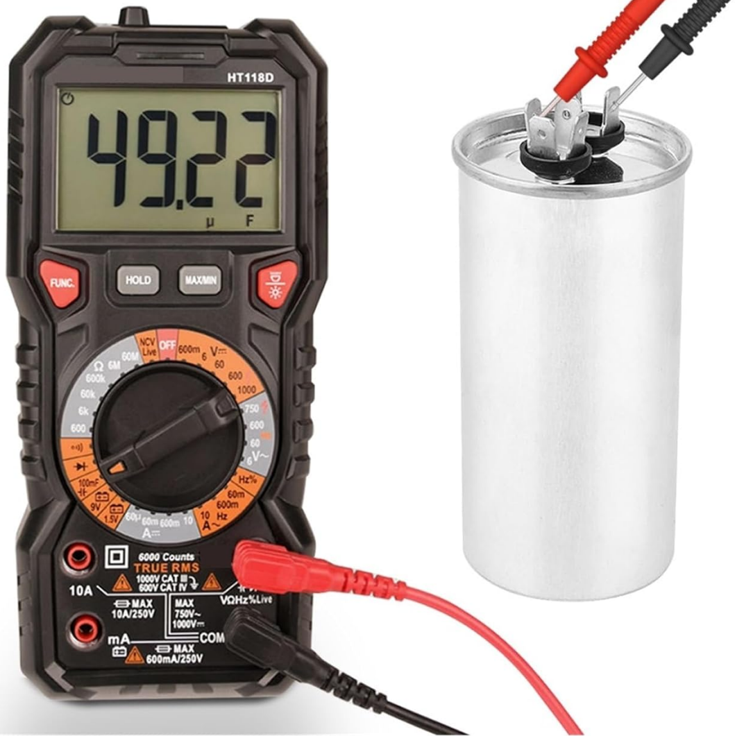
Figure 6.1: The HT118 multimeter displaying a capacitance measurement.
