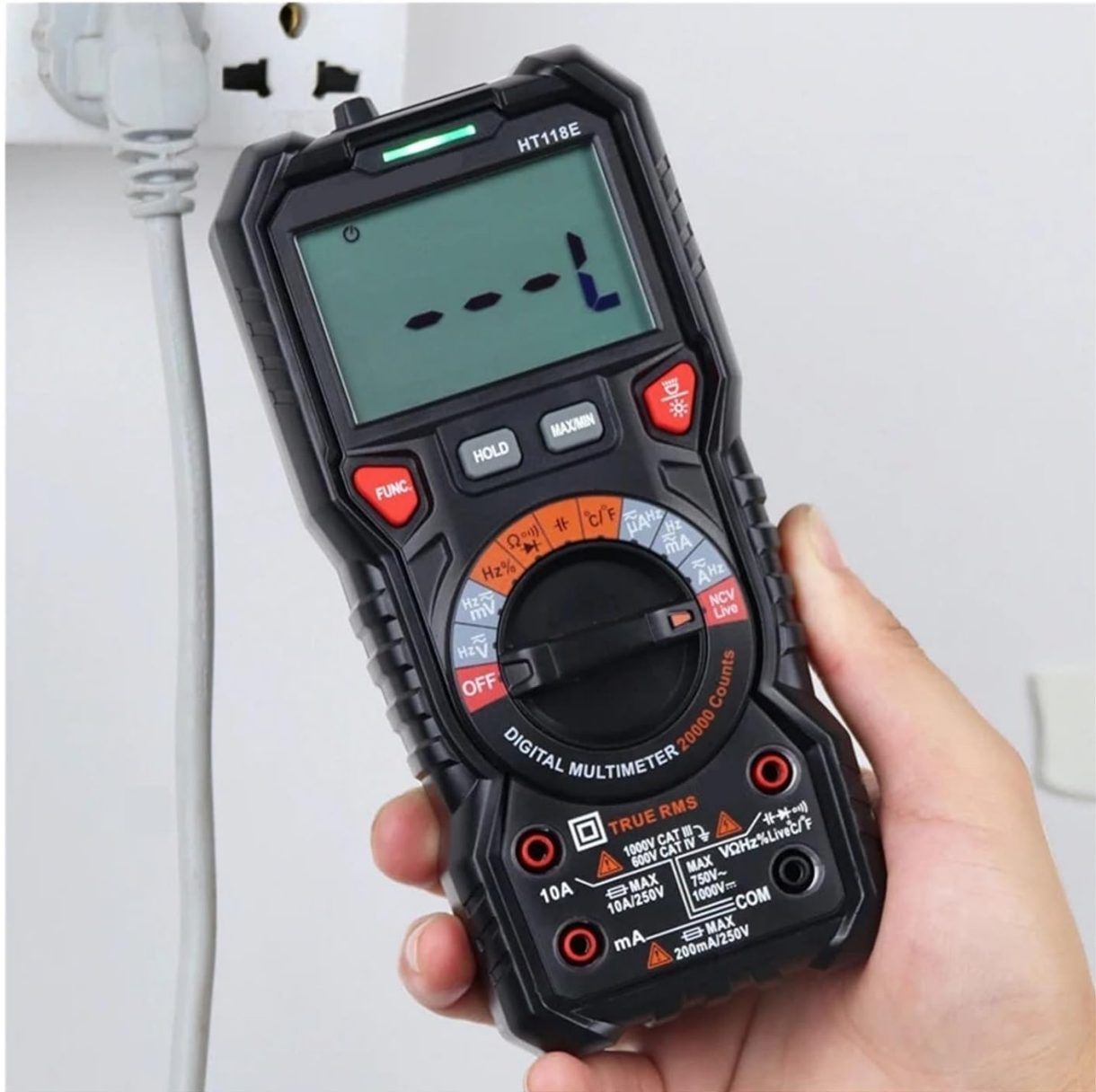
Figure 6.3: The HT118 multimeter displaying "LIVE" during live wire detection.
