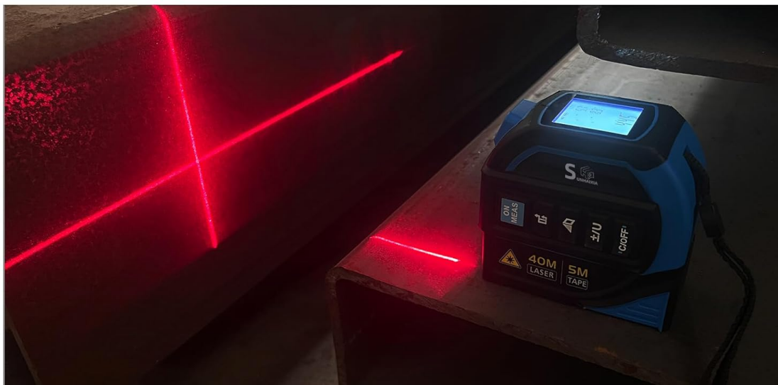
Figure 6: Visual demonstration of the electronic level and laser crosshairs.
