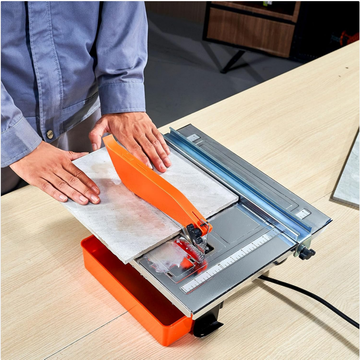
Figure 4.3: Demonstrating the proper technique for feeding material into the saw.
