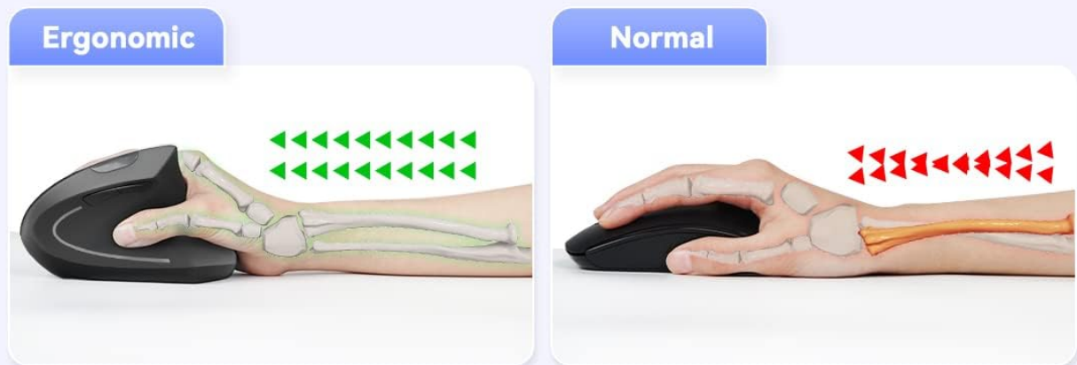
Image: Illustration demonstrating the ergonomic benefits of the vertical mouse compared to a traditional mouse, highlighting reduced wrist strain.
