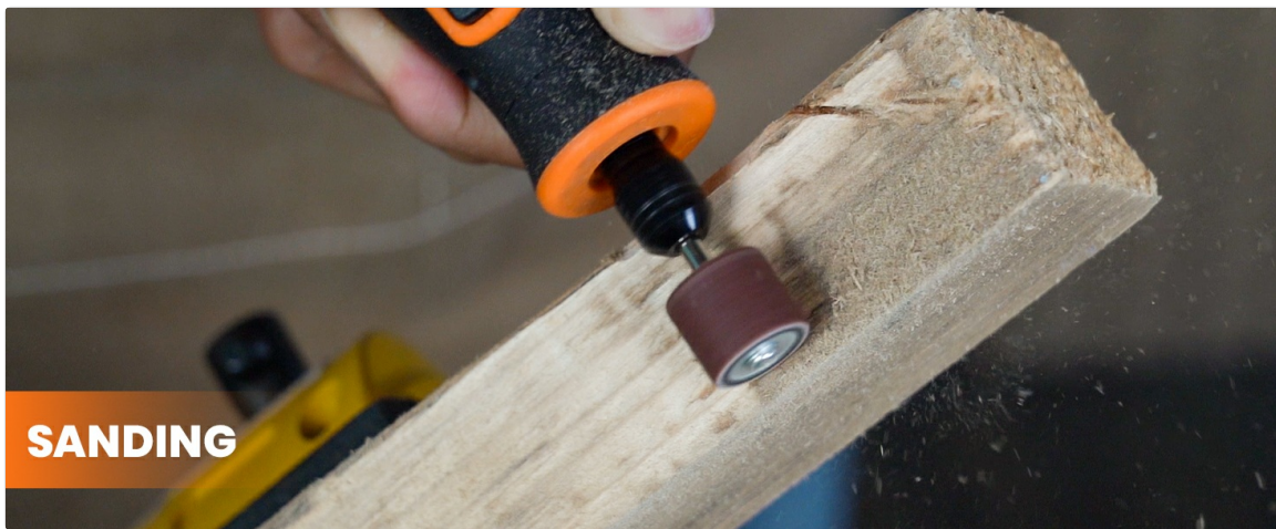
Image 5.4: The rotary tool being used for sanding a piece of wood, showing a sanding band attachment smoothing the surface.
