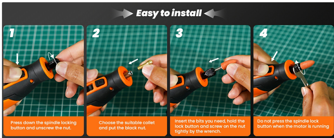
Image 4.2: A visual guide demonstrating the four steps for installing a general accessory: pressing the spindle lock, selecting the collet, inserting the bit, and tightening the nut with a wrench.
