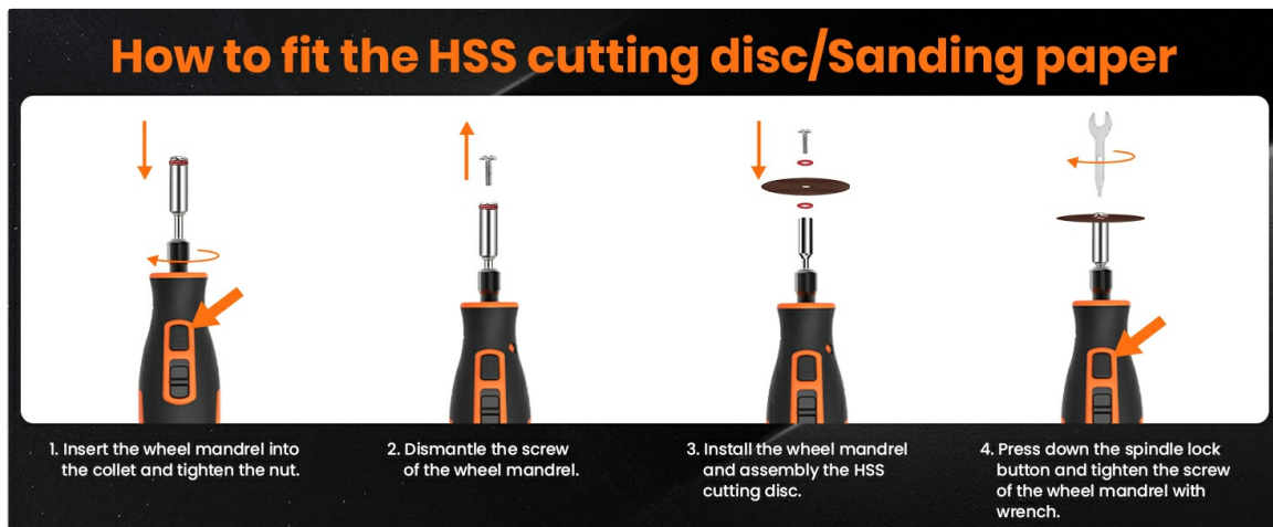
Image 4.4: A visual guide demonstrating the four steps for fitting an HSS cutting disc or sanding paper: inserting the mandrel, dismantling the screw, assembling the disc/paper, and tightening the screw.
