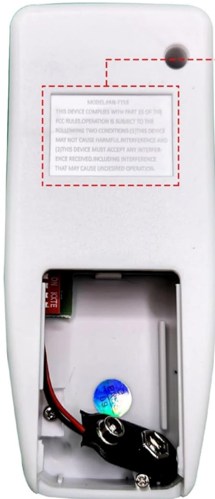
Image 3.1: Diagram showing the location of the FCC ID on the back of the remote and a list of compatible FCC ID/Model numbers for replacement.
