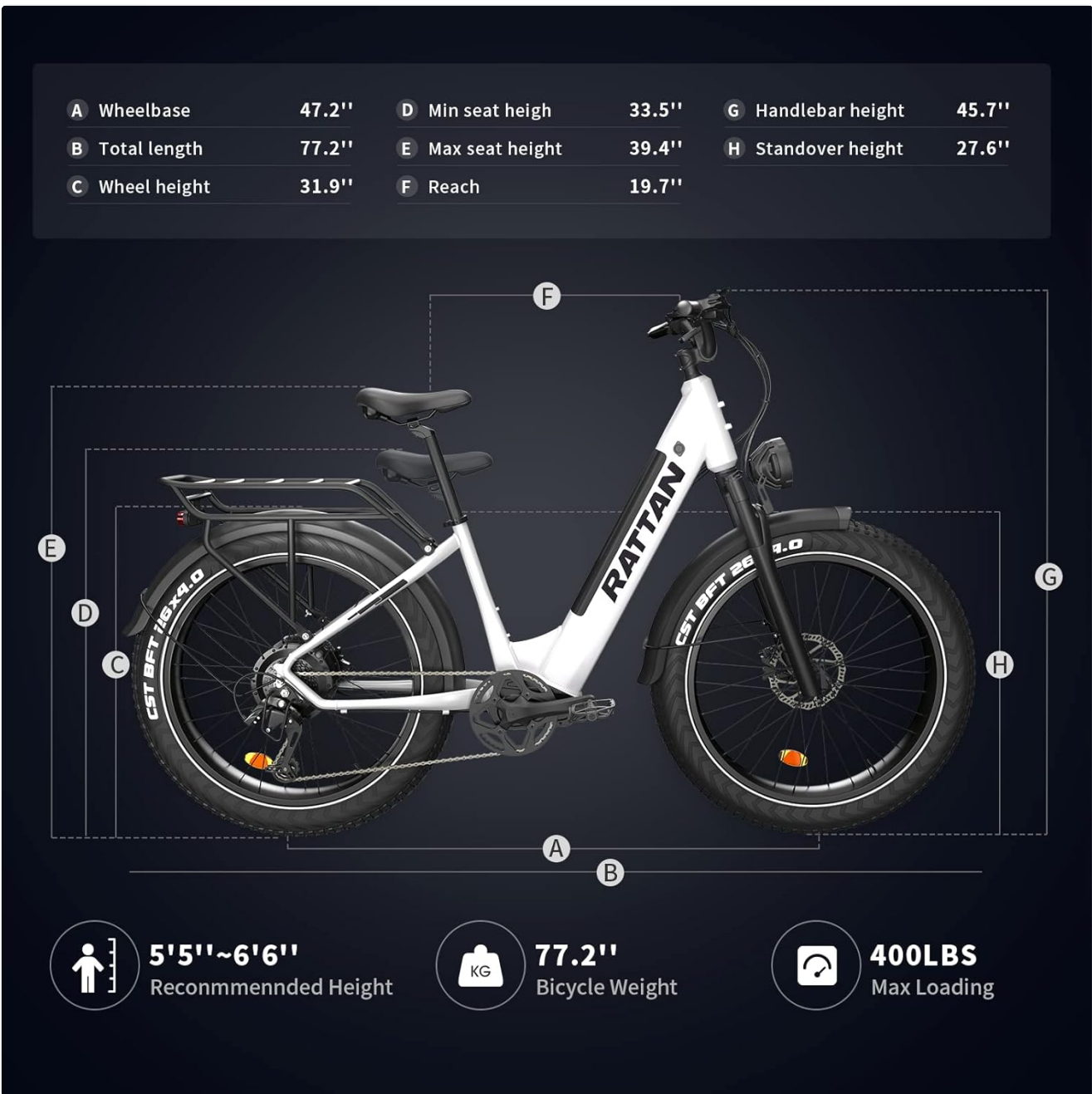
Figure 7.1: Key dimensions and weight of the Rattan Pathfinder Electric Bike.
