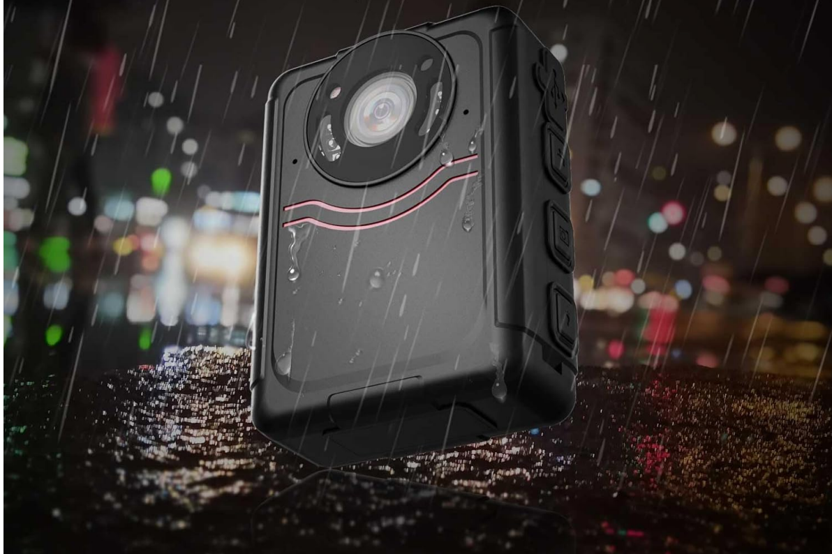
Figure 5: The body camera showcasing its IP65 waterproof design, indicating resistance to water and dust.
