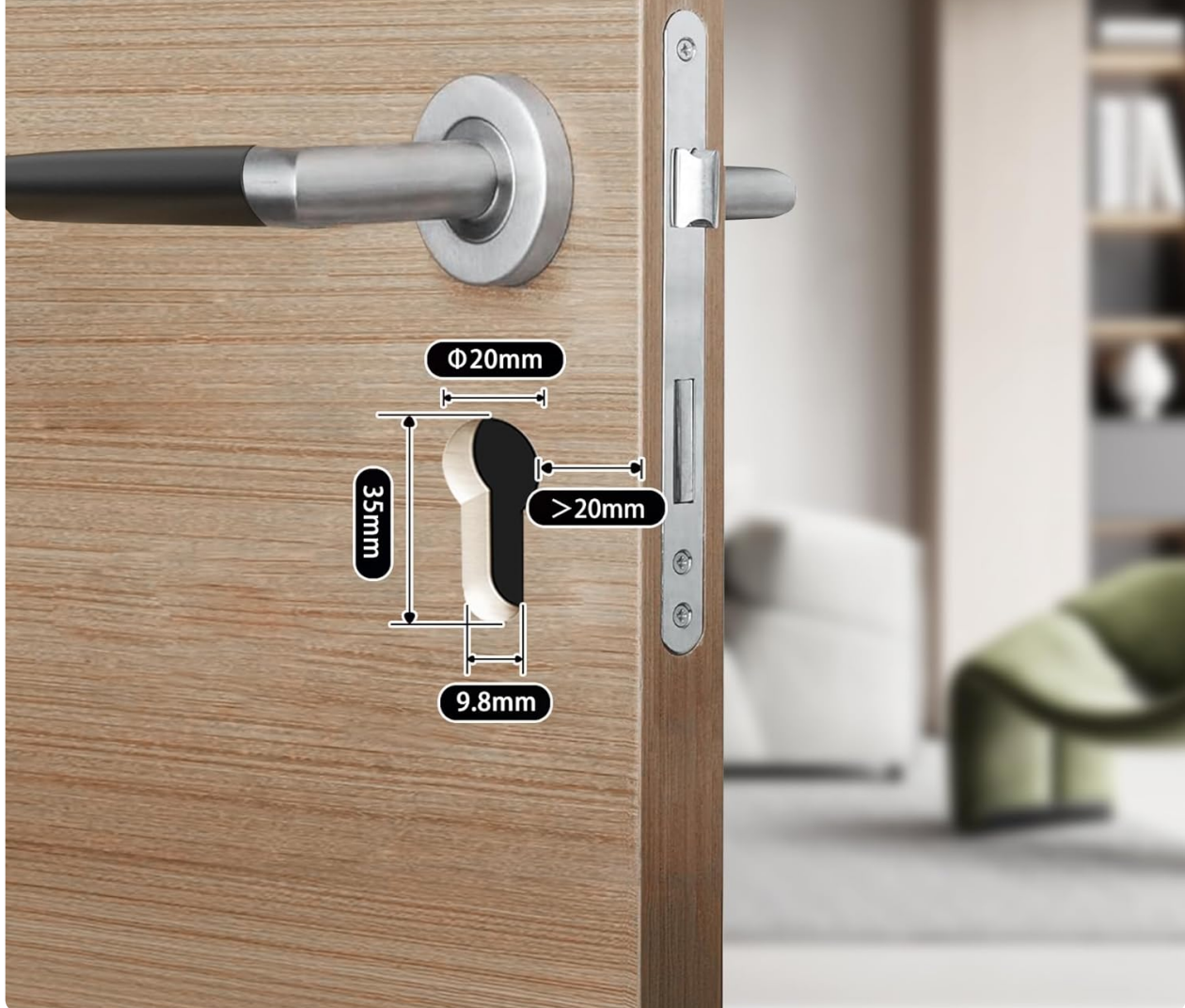
Figure 3.2: Required dimensions for the lock cylinder hole.
