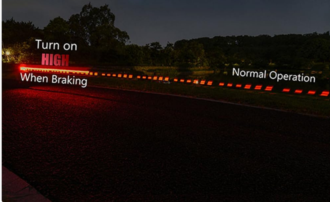
Image: A visual representation of the advanced brake sensing technology, where the taillight intensifies its illumination upon detecting deceleration.
