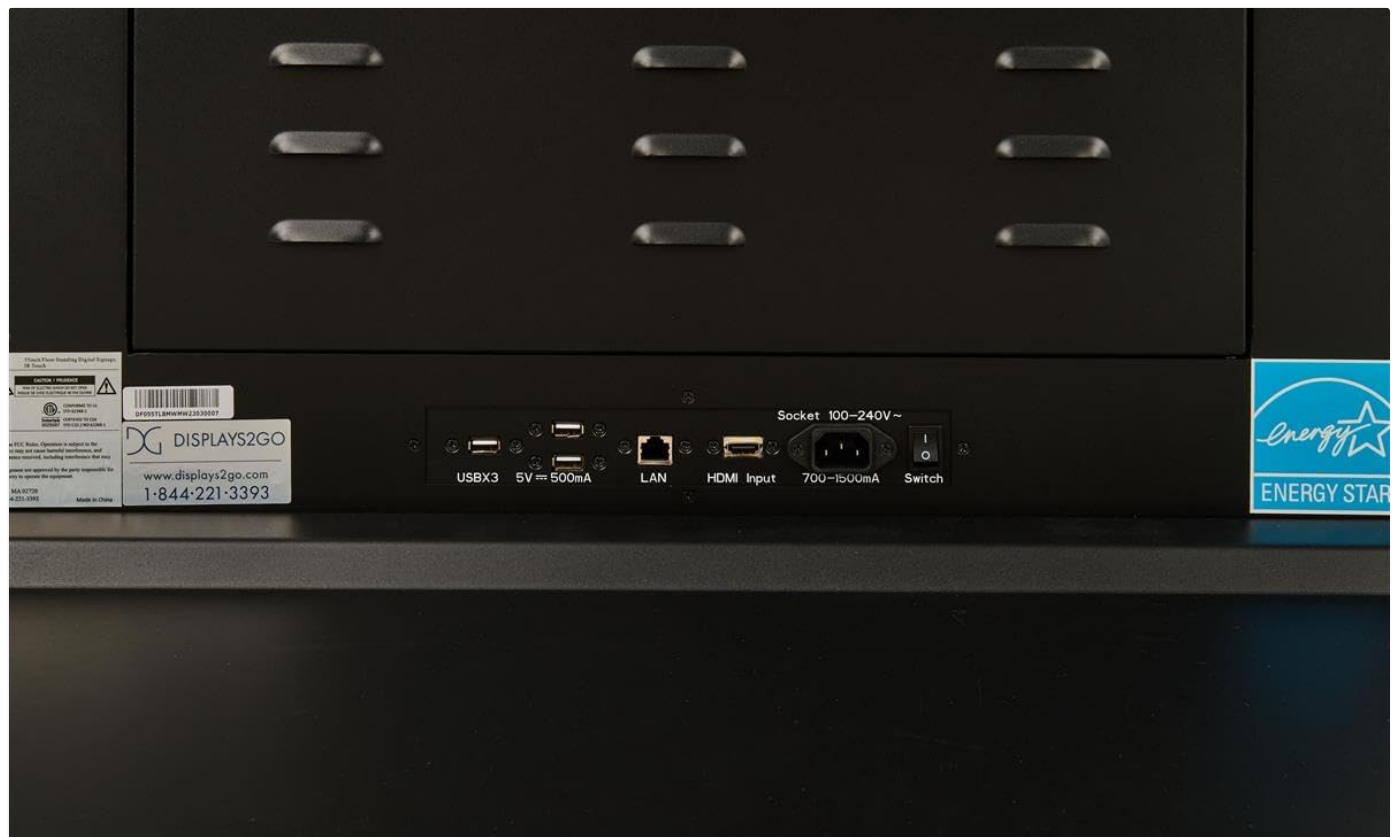
Figure 4: Detailed view of the kiosk's connectivity ports and power switch.
