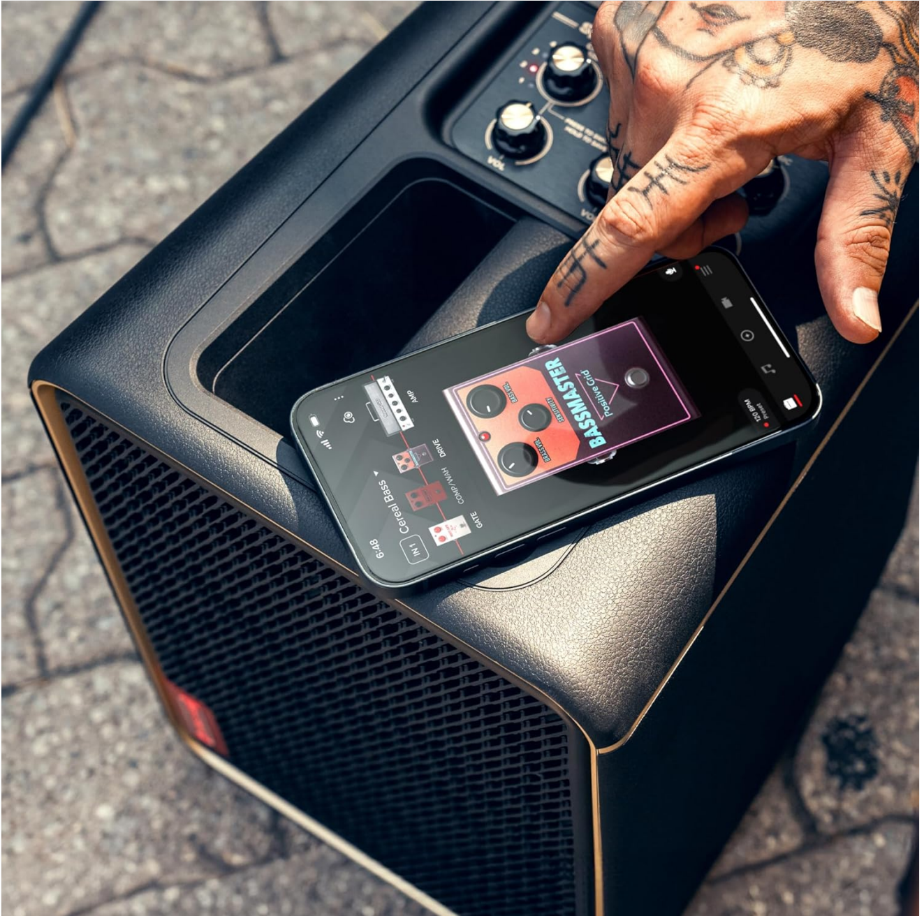
Figure 5: The Spark app interface on a smartphone, demonstrating the ability to control effects and amplifier models directly from the device.
