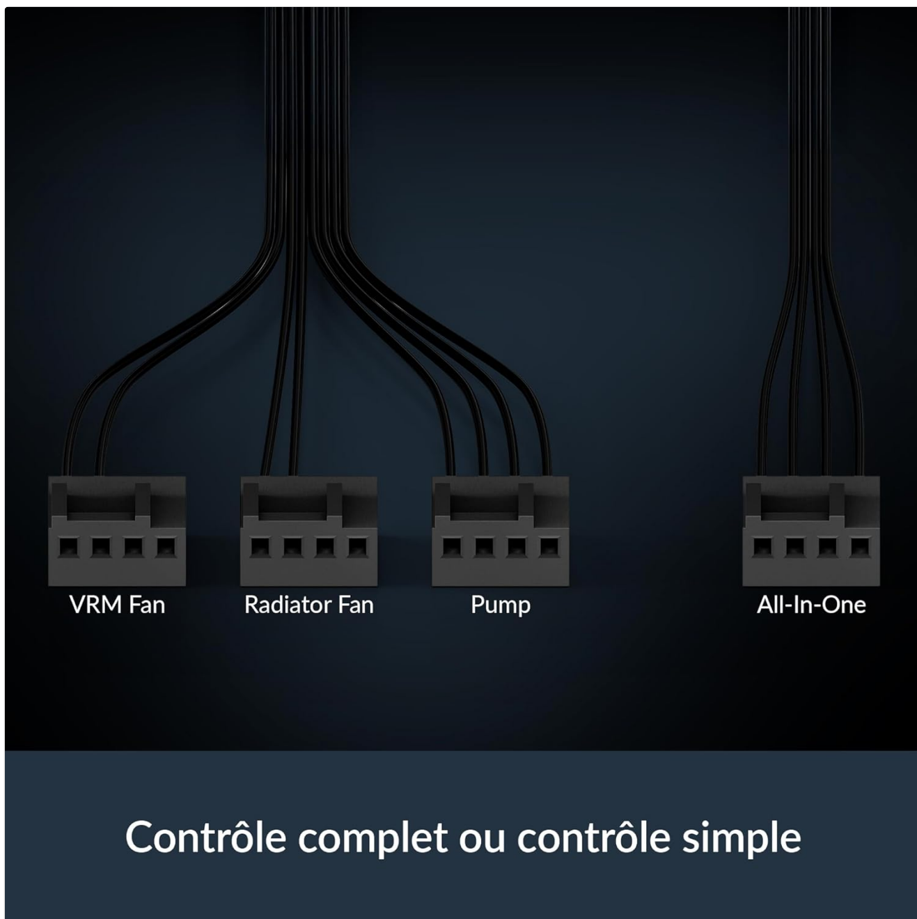
Image: Wiring Options: Diagram showing two wiring configurations: 'Full Control' with separate connections for VRM Fan, Radiator Fan, and Pump, and 'Simple Control' with a single All-In-One connection to the motherboard.
