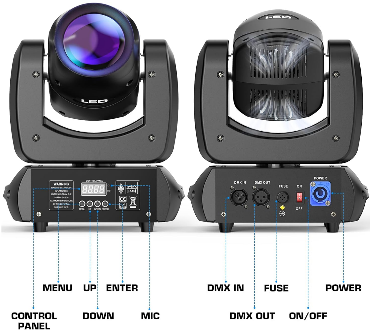
Image 3.4: Control Panel and Connection Ports.
