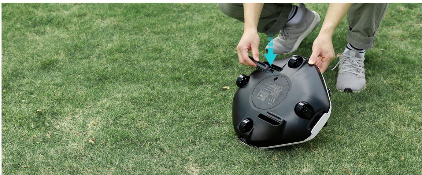
Figure 4.2: Activating the cleaner with one-click before placing it in the pool.
