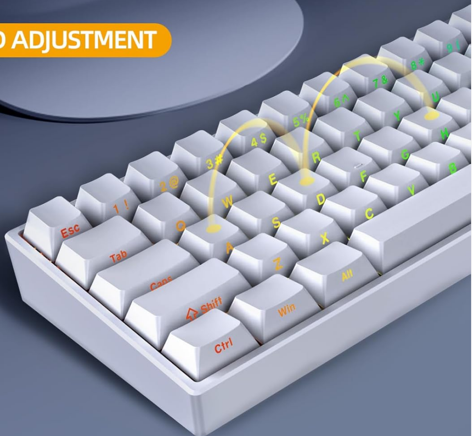
Image: A visual representation of the customizable 200-segment key travel, illustrating the RT adjustment range of 0.02mm-4.0mm and 0 deadband adjustment.
