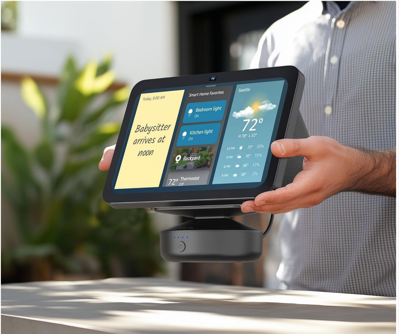
Figure 4.1: Magnetic attachment of the Show 8 3rd Gen to the battery base.
