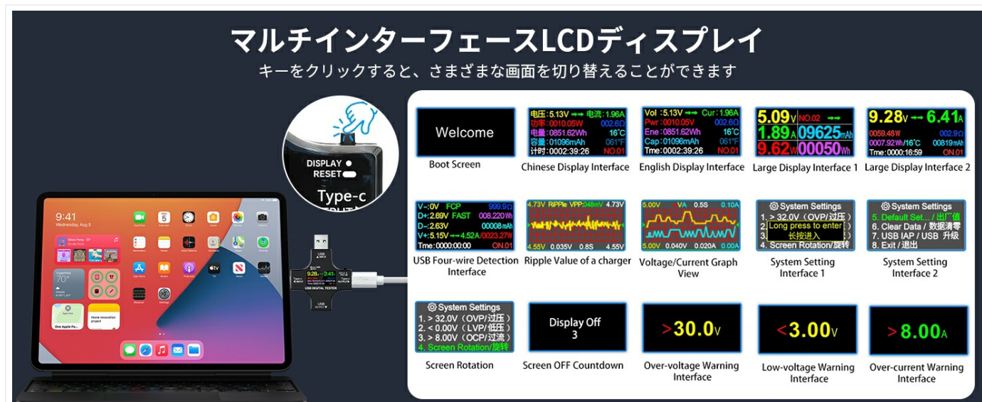
Figure 5: The multi-interface LCD display allows users to switch between various screens by clicking the button.
