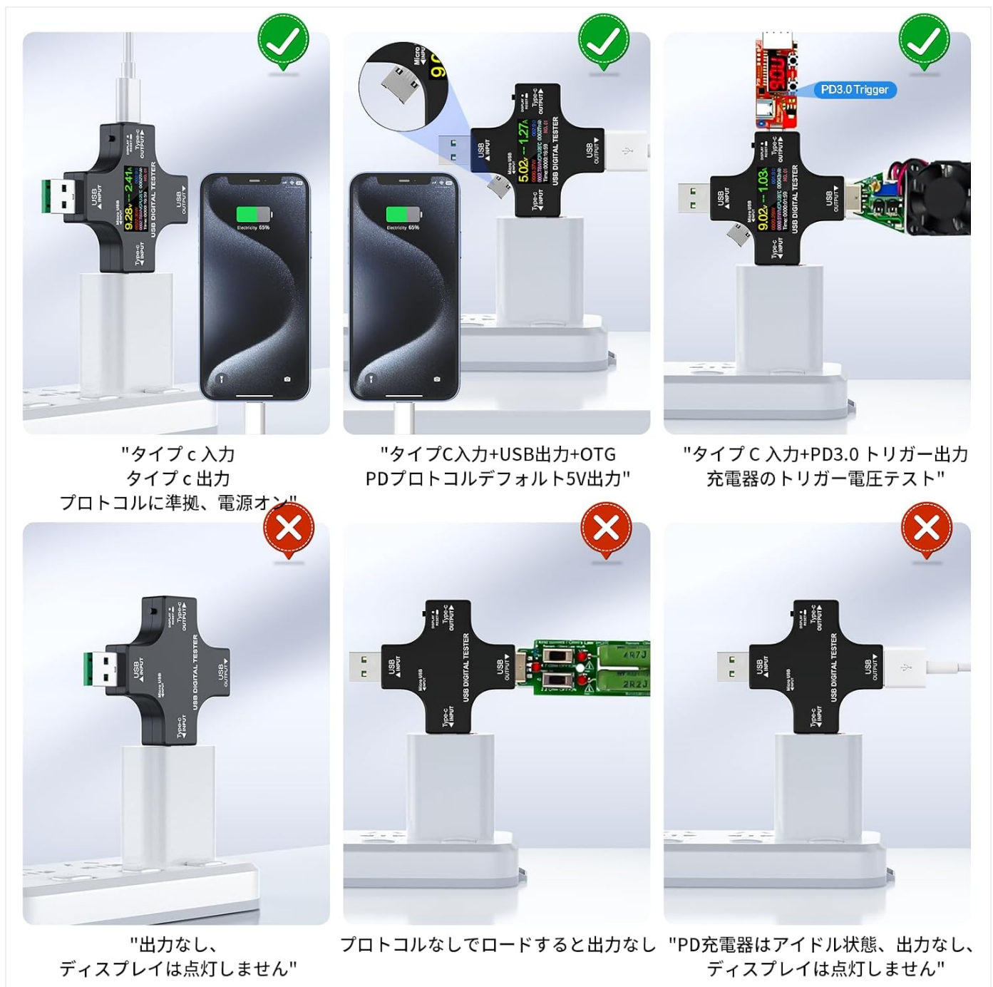
Figure 10: Examples of correct (green check) and incorrect (red X) connection methods, highlighting scenarios where the display may not light up due to lack of output or protocol issues.
