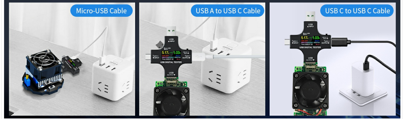
Figure 8: The tester can be used to evaluate the charging speed and quality of Micro-USB, USB-A to USB-C, and USB-C to USB-C cables.
