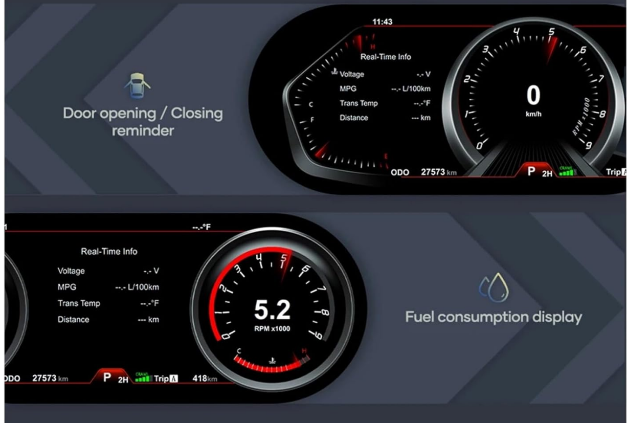
Figure 5.2: Display showing real-time information such as voltage, MPG, transmission temperature, and distance, alongside a door opening/closing reminder and fuel consumption display.
