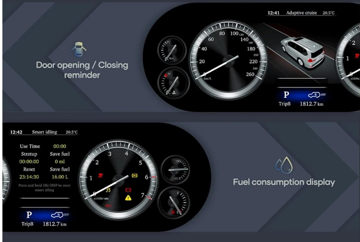
Figure 5.2: Example of the dashboard interface displaying door status and fuel consumption data.
