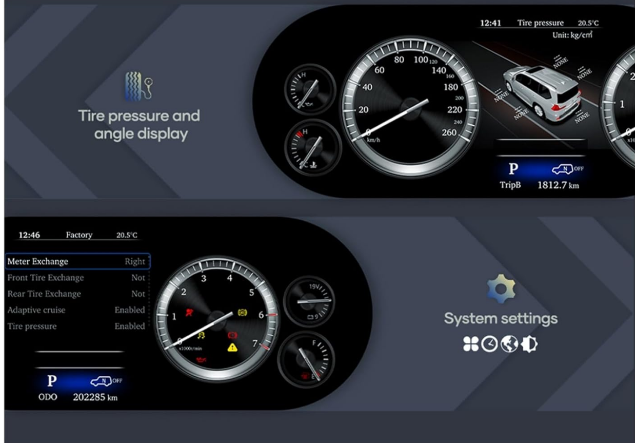
Figure 5.3: Example of the dashboard interface displaying tire pressure and angle, and options for system settings.
