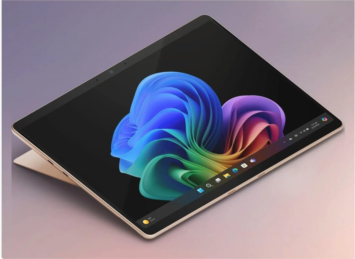
Figure 4.4: Iconic 165-degree fluid kickstand.
