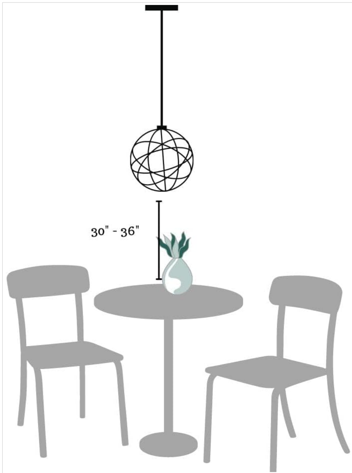
Figure 4: Recommended spacing (30 inches minimum) and height (30-36 inches above surface) for multiple pendant lights over a kitchen island.
