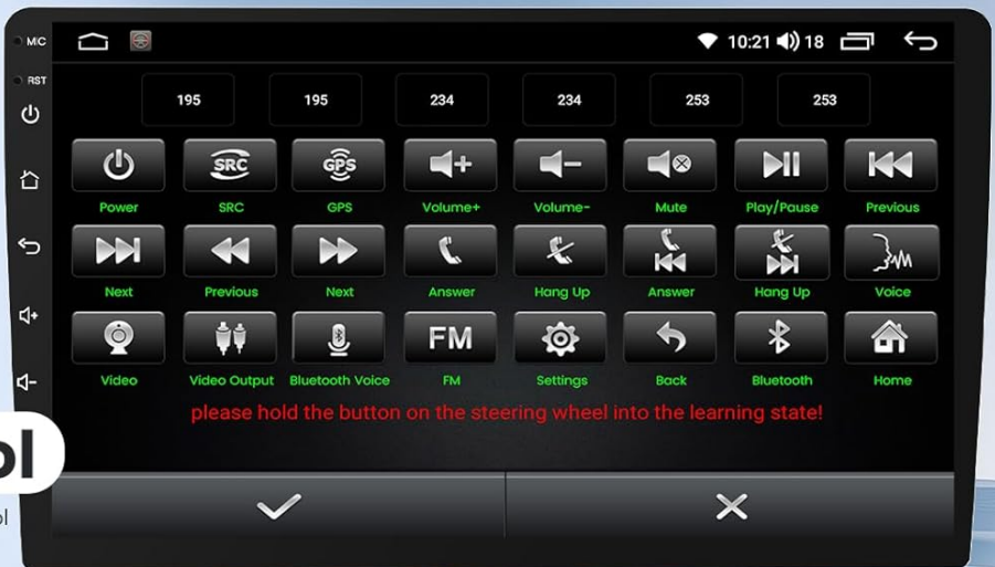
Figure 4.6: The car stereo's interface for programming steering wheel controls, allowing customization of button functions.
