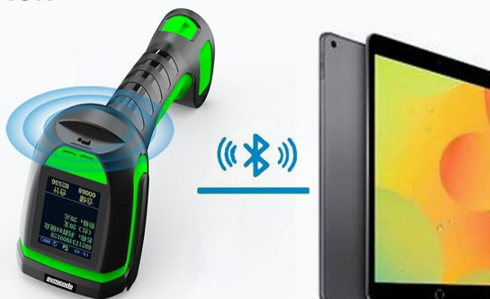
Figure 2.3: Transmission range comparison: Bluetooth (15m/49ft interior) and 433MHz Wireless (600m/1968ft outdoor).
