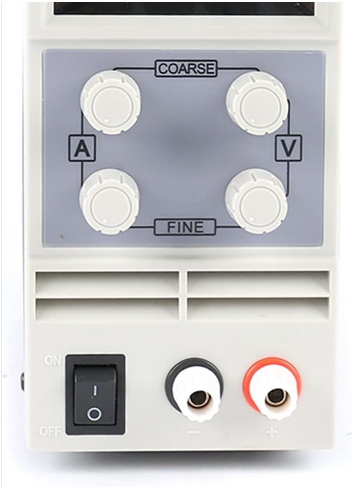
Figure 2: Detailed view of the front panel, highlighting the digital voltage (V) and current (A) displays, coarse and fine adjustment knobs for both voltage and current, the power switch, and the positive (red) and negative (black) output terminals.
