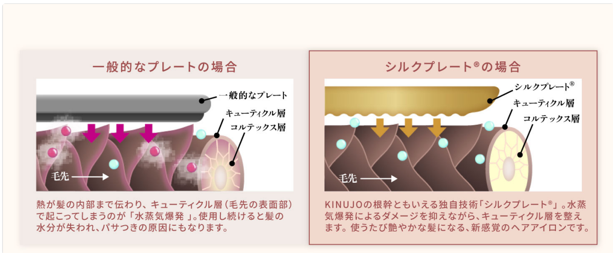
Image 3.2: A diagram illustrating the difference between a general hair iron plate and the KINUJO Silk Plate. The Silk Plate prevents 'steam explosion' by not evaporating water from the hair, thus protecting cuticles and maintaining moisture.
