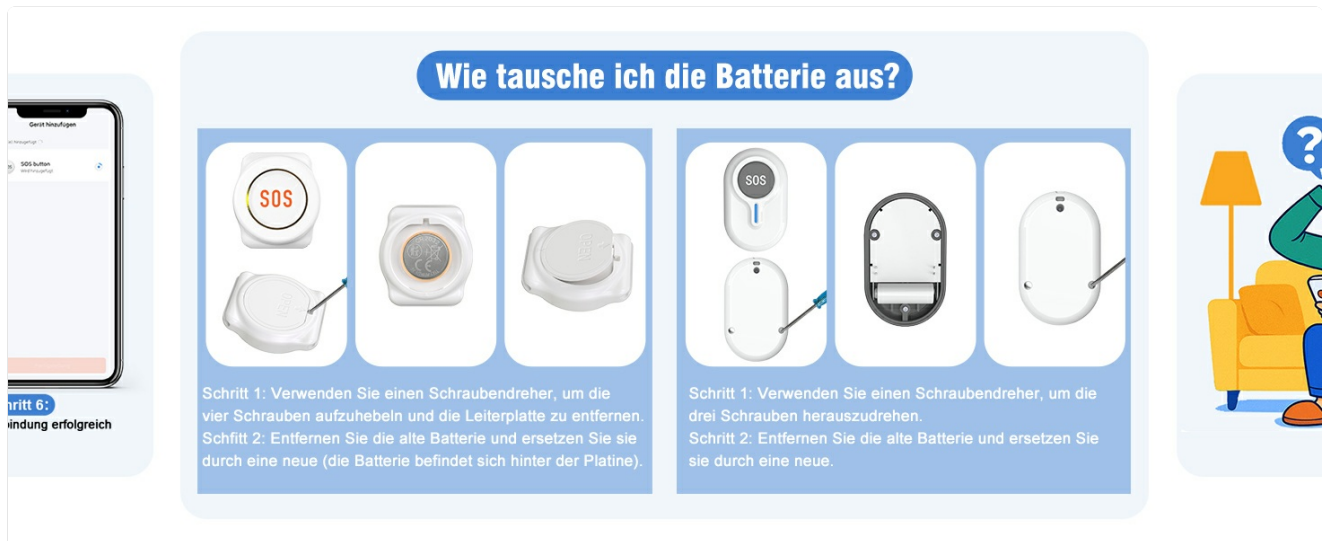
Figure 5.1: Instructions for replacing the battery in the SOS wristband and button.
