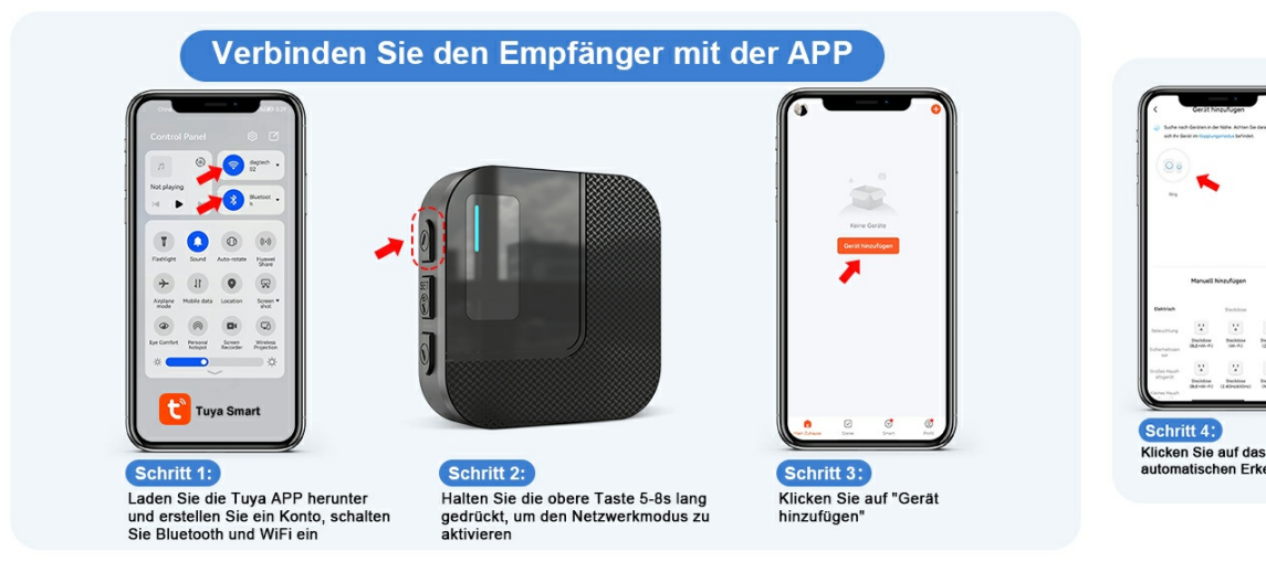
Figure 3.2: Steps for connecting the receiver to the Tuya Smart App.
