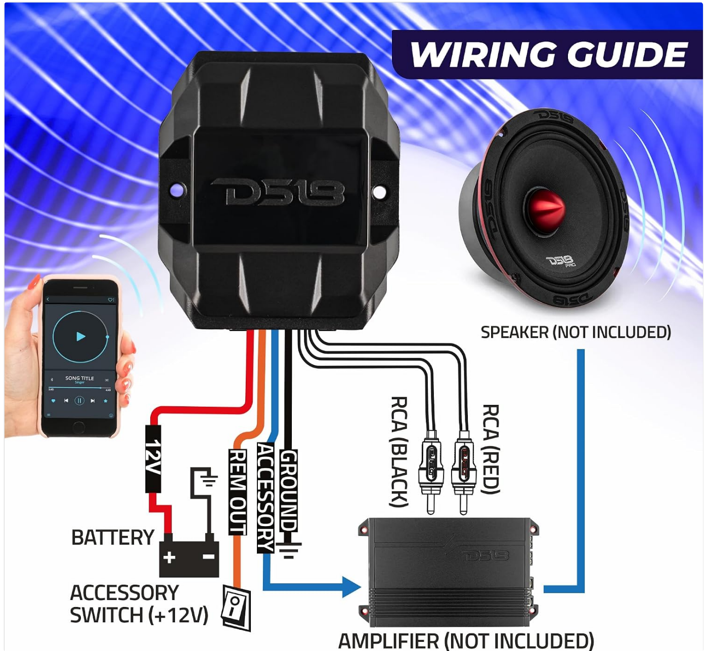
Image: A detailed wiring diagram for the DS18 BTC-Five, illustrating connections to battery, accessory switch, ground, remote out, and RCA outputs to an amplifier.
