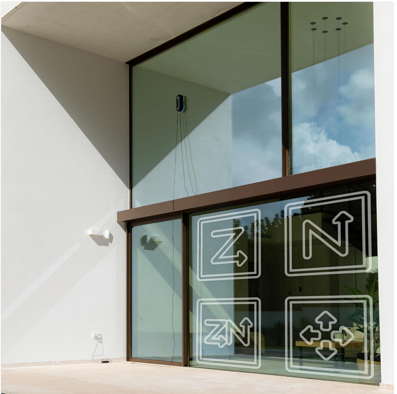
Figure 5.1: The robot illustrating different cleaning path options on a large window.
