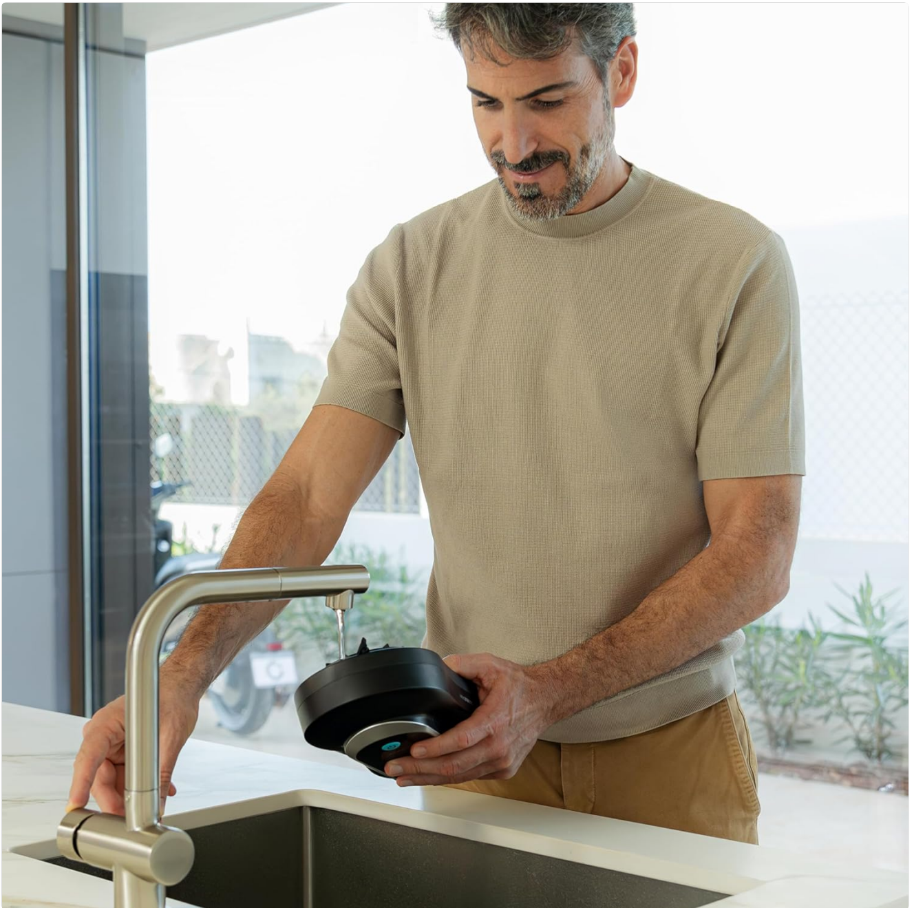
Figure 4.1: A user filling the water tank of the robot window cleaner.
