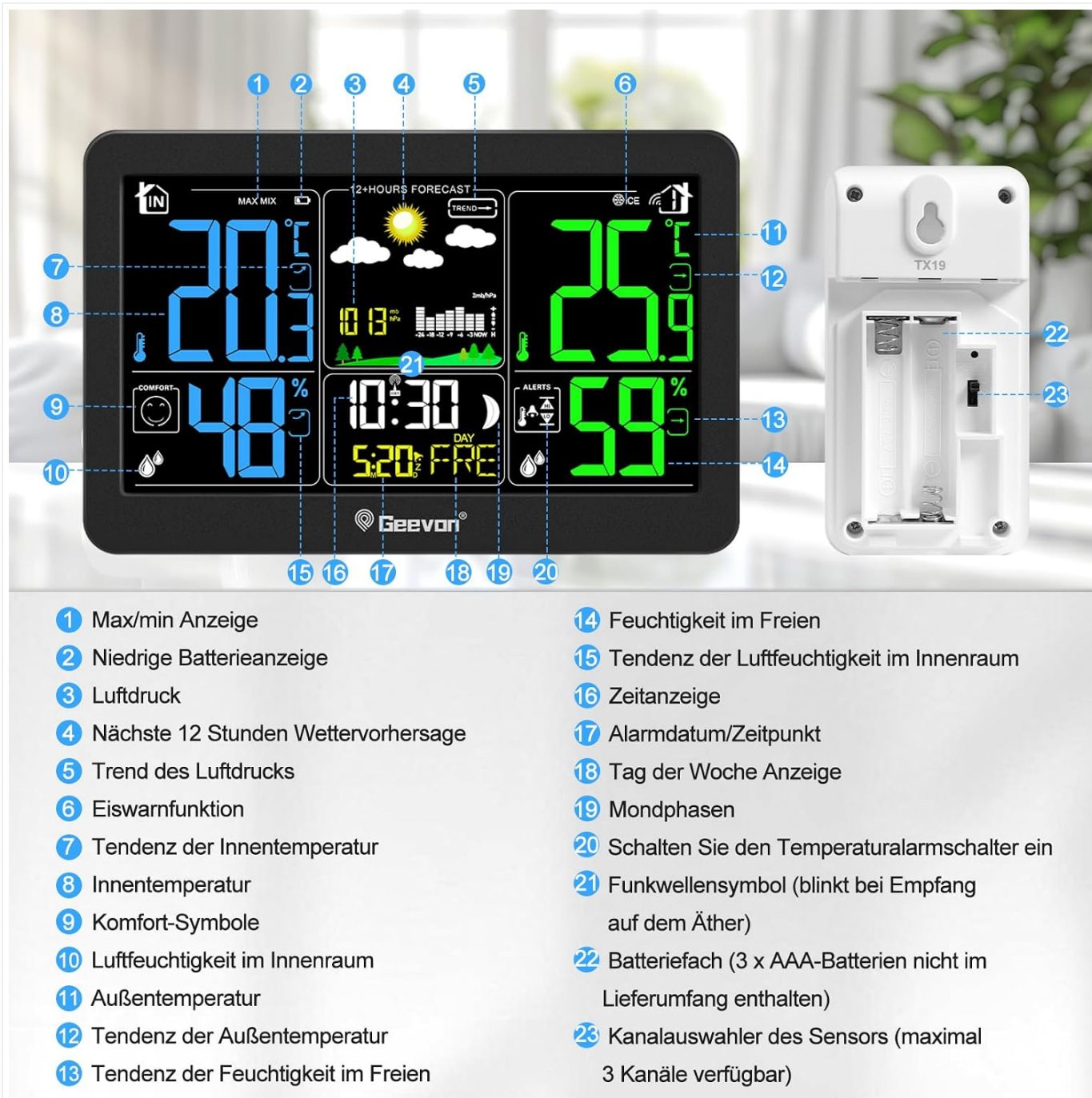
Image: Labeled diagram of the Geevon DCF 246303 weather station main unit and outdoor sensor.
