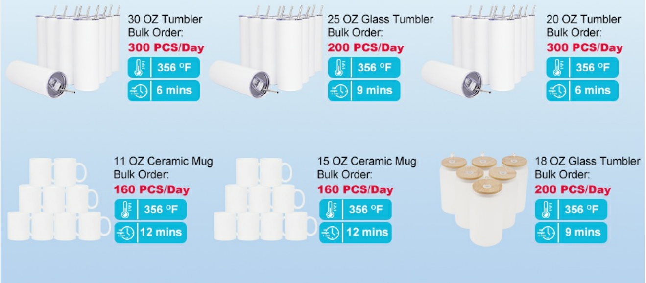
Figure 6: Recommended temperature and time settings for various sublimation blanks.
