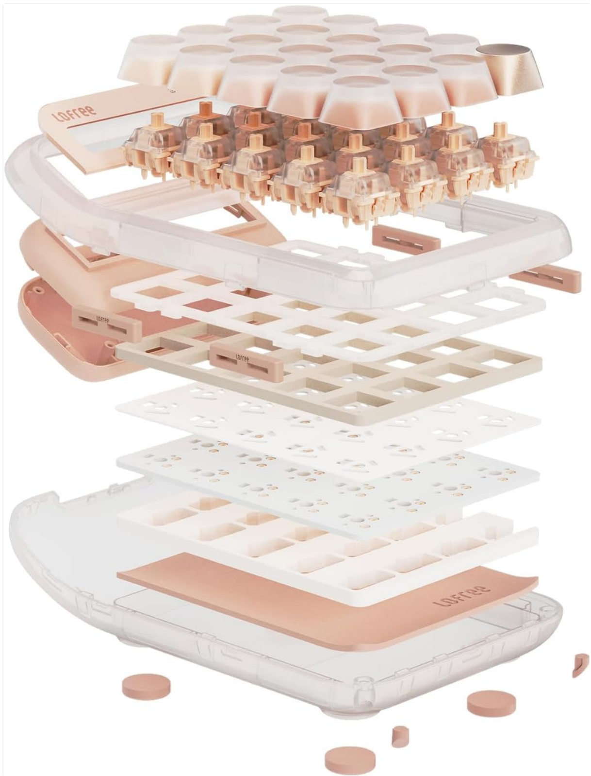
An exploded diagram showing the internal layers and components of the numpad, including keycaps, switches, and circuit board.
