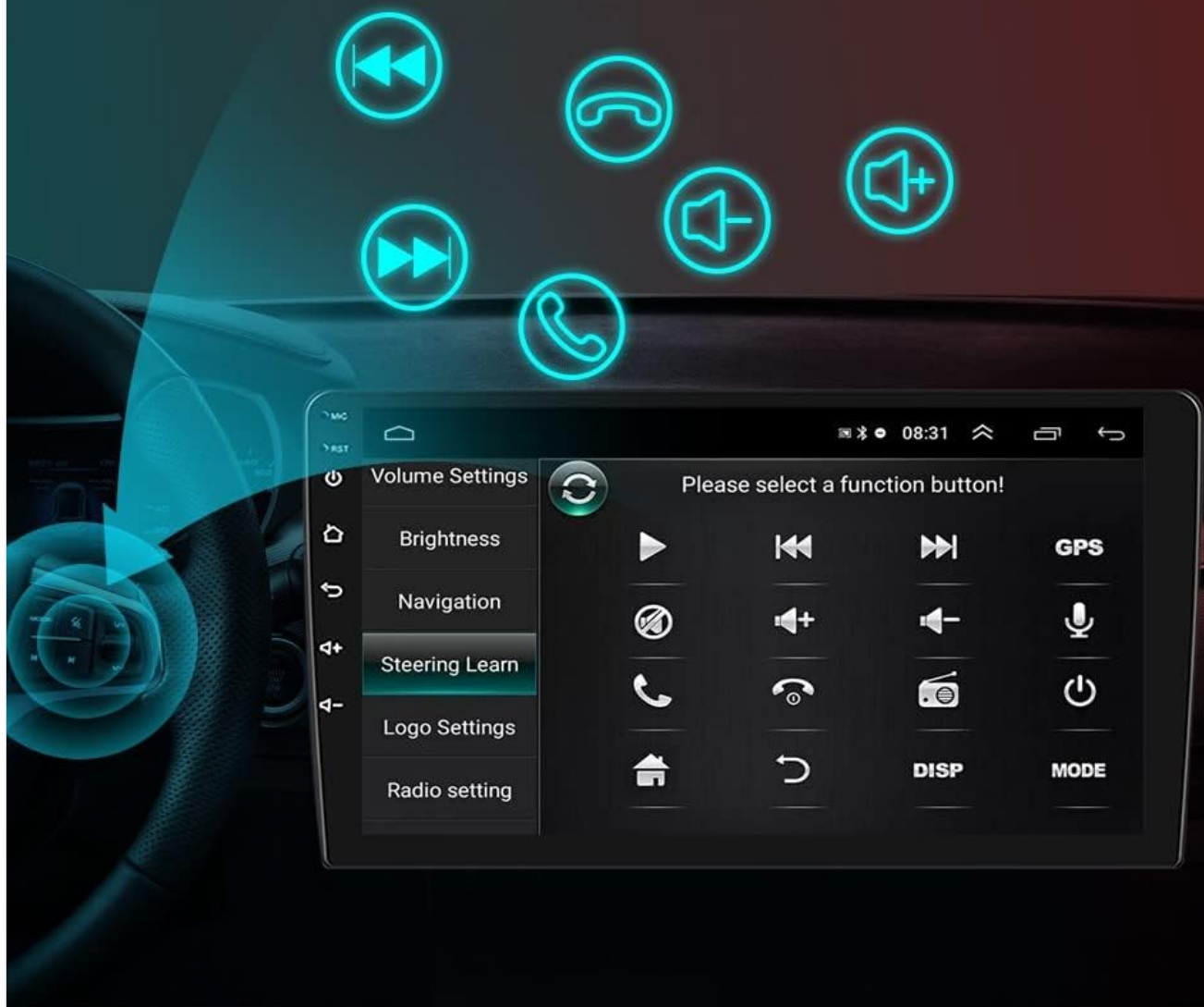
Image 4.6: The steering wheel control learning menu, showing options to assign functions to vehicle buttons.
