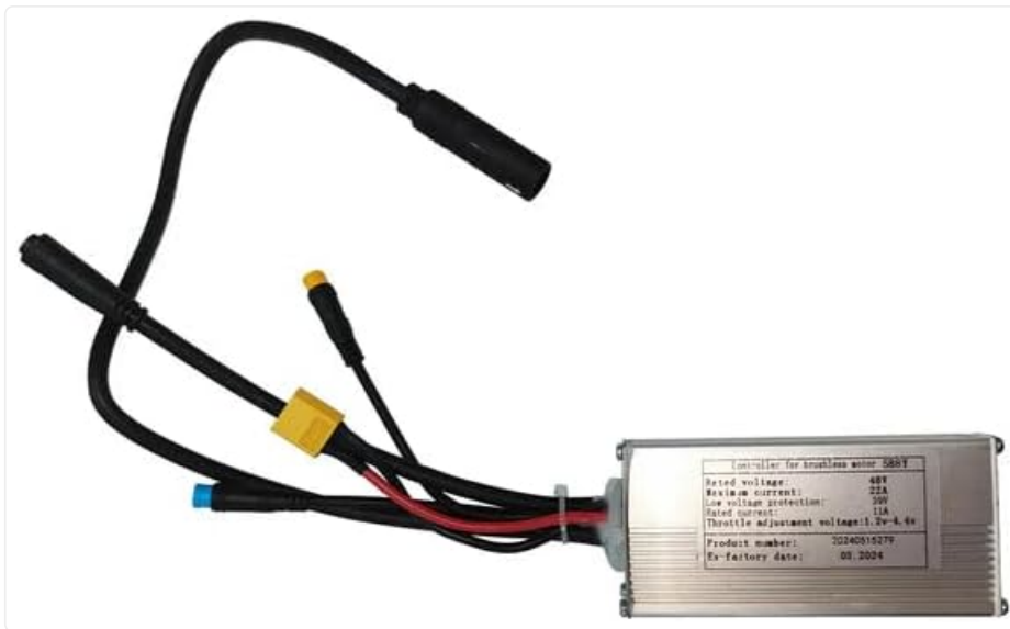
Image 1: The Wildway KW26 Controller, showing its compact metal casing and various color-coded connectors for motor, battery, throttle, and other ebike components.
