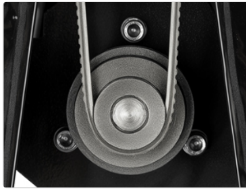
Figure 4.3: Close-up of the belt drive system, illustrating how to change belt positions to select different speed ranges.
