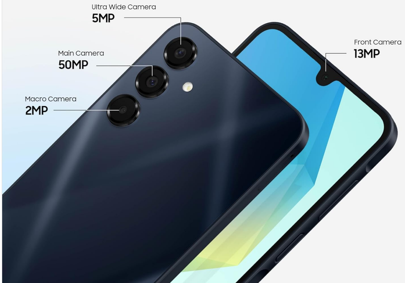
Figure 3: Overview of the Galaxy A16 5G camera system.
