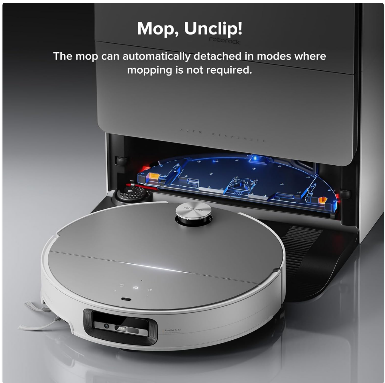
Figure 5: The robot detaching its mop pad at the dock.
