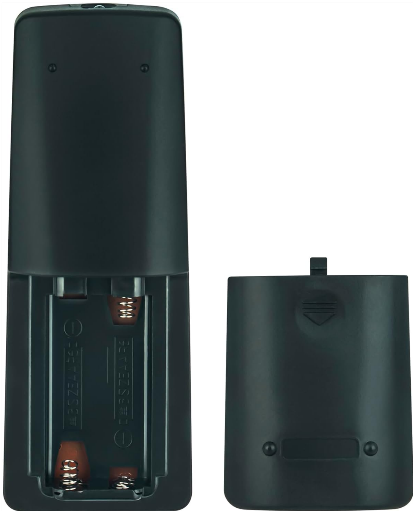
Figure 2: Open battery compartment showing correct battery orientation.
